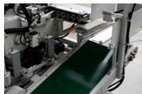
传送带式收料装置 Conveyor-type receiving device
