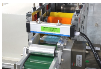
平面切片 Flat mask cutting
