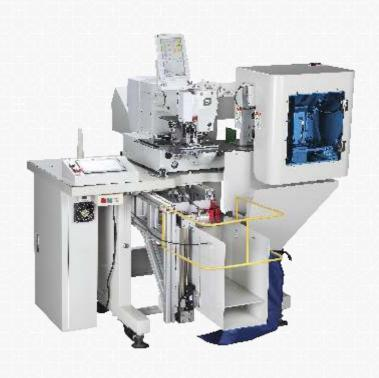
机器使用范围主要用于T桖衫拼圆领,以及袖口类似工艺 The machine is mainly used in the T-shirt with crew neck, and the similar process of cuffs
